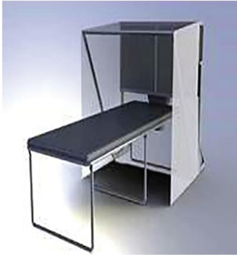
**Figure 1** Ventilating headboard. The ventilating headboard consists of lightweight, sturdy and adjustable aluminium framing with a retractable plastic canopy. It is fitted with a high-efficiency particulate air fan/filter unit for filtration (adapted from Mead<sup>48</sup>).
