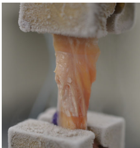
Figure 4. Tendon construct testing with an all-electric dynamic test load system.
