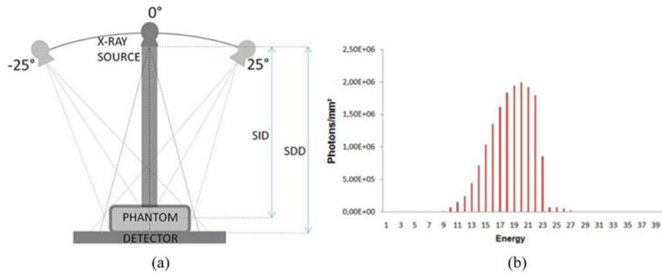
**Figure 3.** Simulated BT and 2D mammography acquisition geometry: (a) schematic representation of the acquisition system (b) simulated 28 kVp W/Rh mammographic spectrum.
