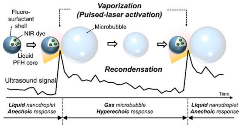
**FIG. 1.** Vaporization and recondensation of laser-activated nanodroplets (LANDs) in response to an optical trigger. When activated, LANDs immediately produce strong ultrasound signals, which decrease as the LANDs recondense to native, liquid droplets.
