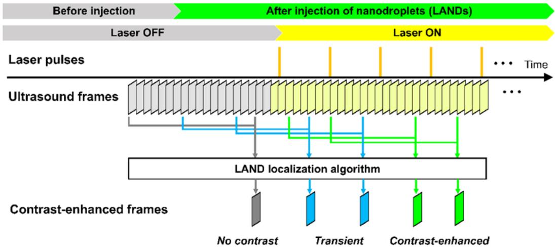
**FIG. 2.** An imaging configuration for the localization of LANDs. After both injecting and triggering LANDs, this algorithm can reconstruct contrast-enhanced LAND image frames at the pulse repetition frequency of a laser system.
