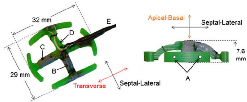
**Fig. 1.** Developed mitral annular force transducer with measurement directions and features identified: (A) suture passages for transducer-annulus anchoring, (B) strain gage to measure septal-lateral force, (C) strain gage to measure transverse force, (D) transducer spring element, and (E) exit wire harness.
