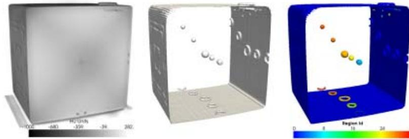
Fig. 3. Effect of different image analysis filters used to automate the QA process. The first picture (a) shows a volumetric representation of the CT scan of a Modus phantom. Phantom features (b) are detected using a contouring algorithm with a HU threshold of -500. To select individual features, a labeling algorithm is used. The output of the algorithm is color-coded in (c), where each individual phantom feature is represented using a different color.
