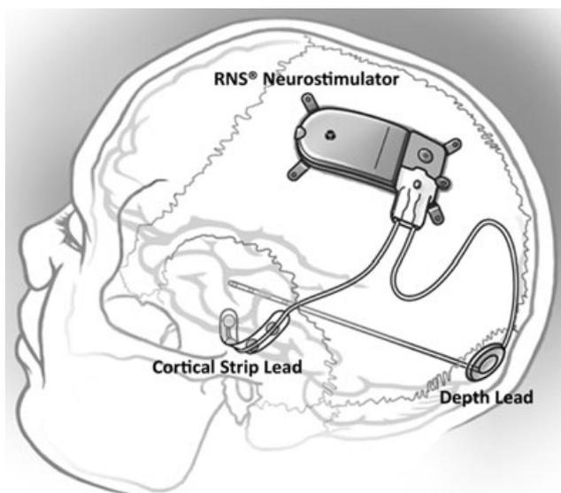
**Figure 1.** Implanted RNS Neurostimulator and NeuroPace Depth Lead and NeuroPace Cortical Strip Lead.
