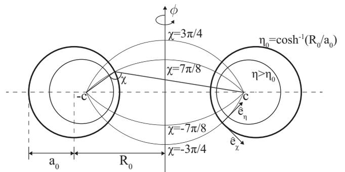
**Fig. 2.** Schematic of the cross-section of a torus illustrating the set of toroidal coordinates,  $\eta$ ,  $\chi$  and  $\phi$ , used in the calculations. The unit vectors,  $\hat{e}_\eta$  and  $\hat{e}_\chi$ , as well as the central-circle radius,  $R_0$ , and the tube radius,  $a_0$ , are also shown.
