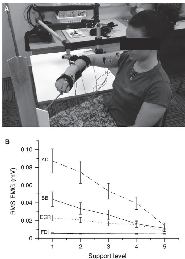
**Figure 1.** (A) Example of experimental arrangement. (B) Background muscle activity as a function of support level, ranging from minimal support (1) to full support (5). Average root-mean-square EMG of anterior deltoid (AD), biceps brachii (BB), extensor carpi radialis (ECR), and first dorsal interosseous (FDI) muscles from the prestimulus interval. Error bars represent  $\pm$  SEM.
