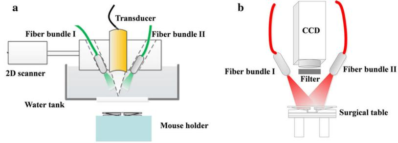
**FIG. 1.** Schematic of the **a** PAI system and **b** NIR fluorescence imaging system. *PAI* photoacoustic imaging, *NIR* near-infrared
