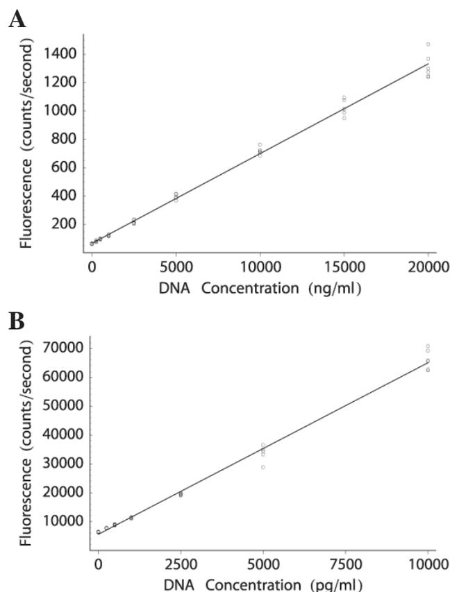
Figure 1. Measurement of high concentrations of DNA (0-20  $\mu$ g/ml). The graphs show the observed data with the linear regression models for the relationship between DNA concentration and observed fluorescence enhancement. Statistical analysis confirms the validity of each model and suggests that ethidium bromide can distinguish smaller differences in DNA concentration than Hoechst 33258 in this range (Table 2A). **A:** Ethidium bromide. **B:** Hoechst 33258.
